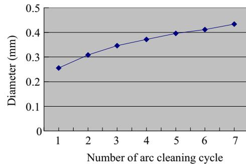
**Figure 4.** The relationship between the spherical tip diameter and the number of arc cleaning cycles; arc power: 230, cleaning arc power offset: 230, cleaning time: 6000 μs.
