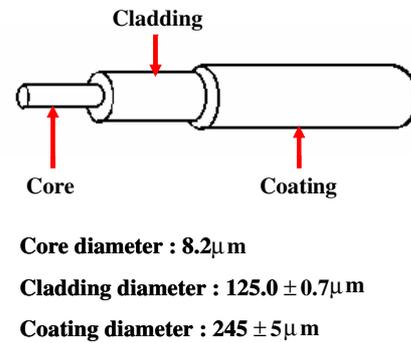
**Figure 1.** The composition and dimensions of a single mode optical fibre.
