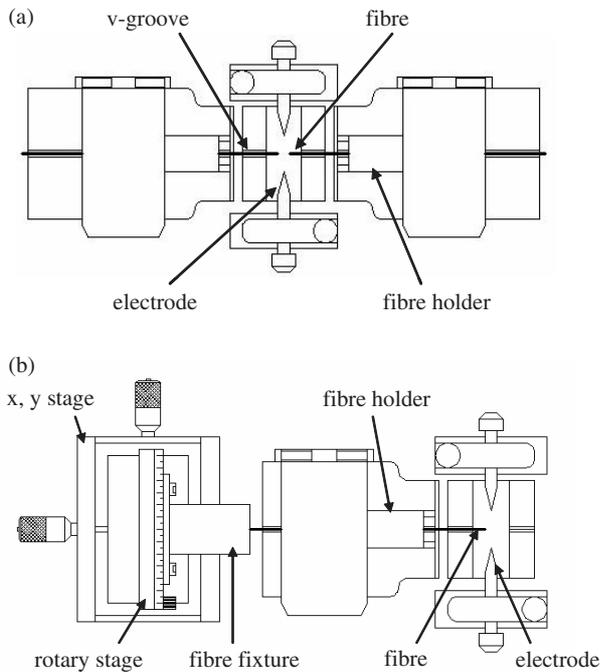
**Figure 2.** Experimental set-up. (a) Original fibre splicer configuration. (b) Modified experimental configuration.
