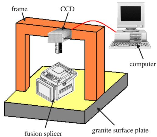
**Figure 3.** The in-process spherical probe forming system.
