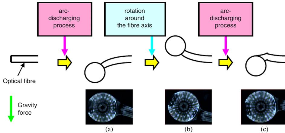
Figure 5. Overcompensation phenomenon (side-view images).
